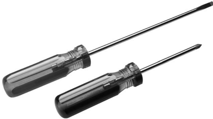
Figure 1.2 Typical screwdrivers, with steel shaft and polymer (plastic) handle.
